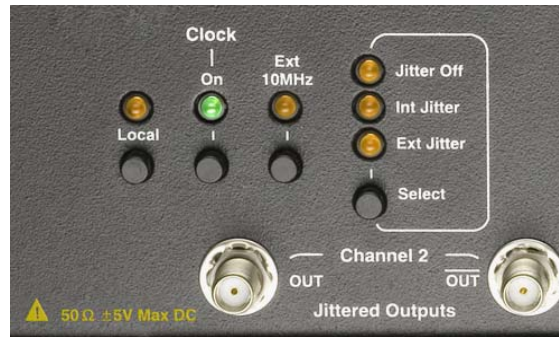
Figure 9 – TG1C1-A front panel – local, receiver, and data path controls
