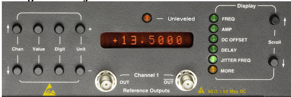
Figure 11 – TG1C1-A front panel – configuration adjustment controls
