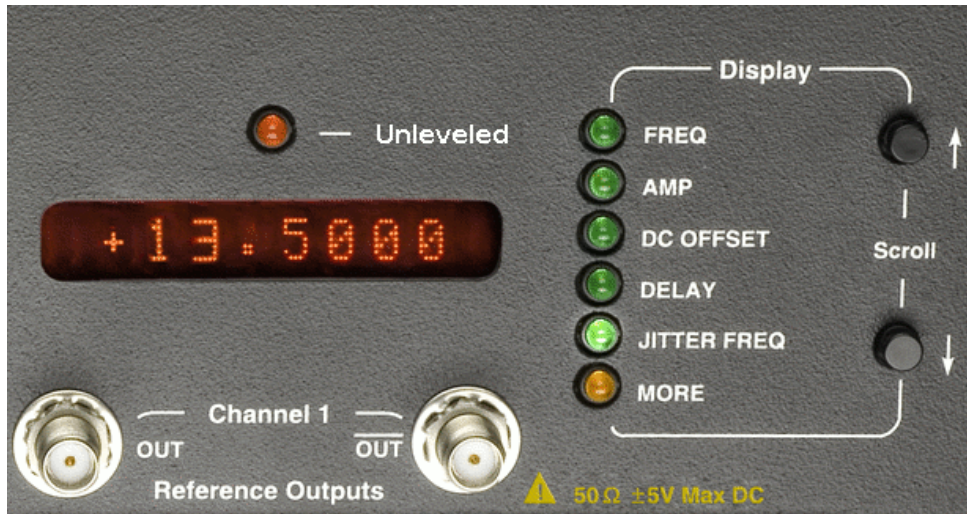
Figure 10 – TG1C1-A front panel – display selection controls
