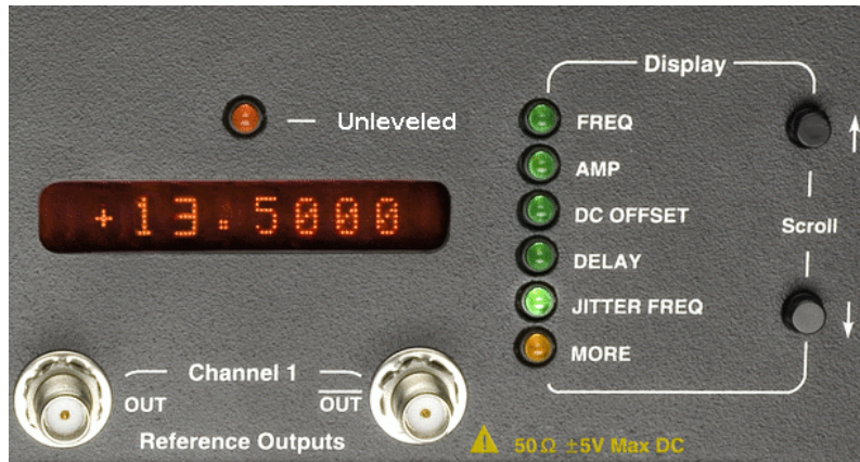
Figure 8 – TG1C1-A front panel – display panel
