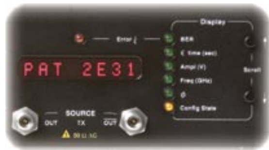
Select from a range of PRBS patterns: from the short 127-bit PRBS7 to the 2-billion bit PRBS31.
